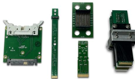
Fig 2. From left to right, two different breakout board types followed by three different loopback schemes.
